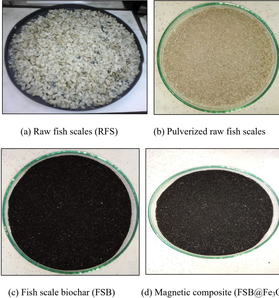
Figure 2.1: The raw fish scales, pulverized fish scales, fish scale biochar and magnetic composite
